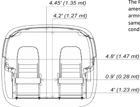
The P2012 cabin has 9 single seats, each with the same amenities (dedicated window and reading light, USB port, armrest, cup holder, fresh air / hot air outlets) and the same generous pitch of a liner's business cabin including air conditioning, venting, and heating for all climate capabilities.
