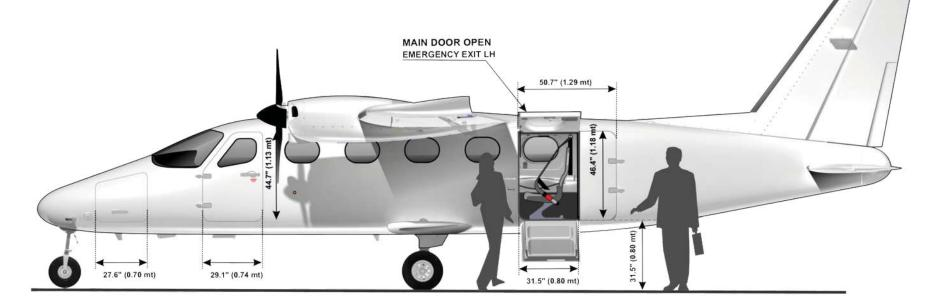
THE FUSELAGE HAS TWO CREW DOORS FOR SEPARATE FLIGHT DECK ACCESS AND A WIDE CABIN DOOR ALLOWING COMFORTABLE PASSENGER BOARDING, FAST CARGO LOADING, SAFE MEDICAL OPERATIONS AND EASY PARA JUMPING. A SEPARATED NOSE COMPARTMENT ALLOWS ADDITIONAL CARGO CAPABILITY. RESPONDING TO THE LATEST CERTIFICATION REQUIREMENTS, NO OTHER AIRCRAFT HAS ALL THESE EXCLUSIVE FEATURES.
